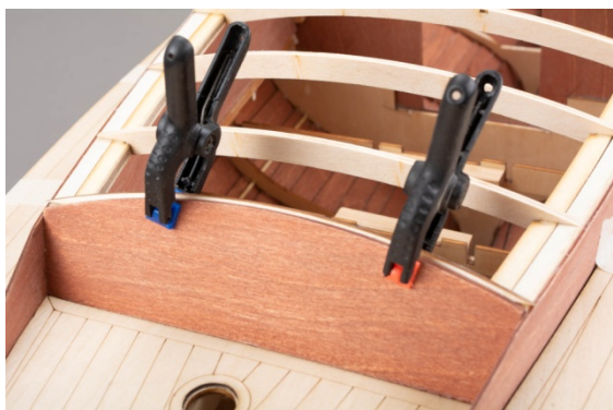
Fig.: Gluing in roof frame 3.17
